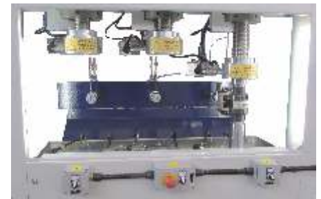
Option for automatic 1/4 turn valve actuator.
