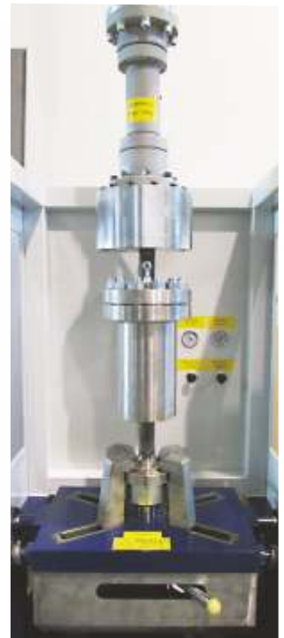
Auto centering claws movement with manual lever
