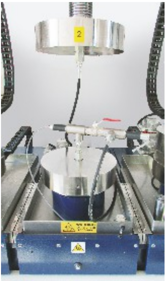
Optional quick clamping for screwed ports valves.
