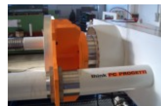
Pressing cylinder with proportional control.
