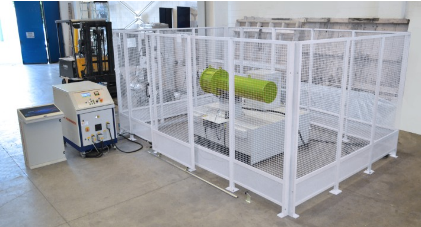
Light perimeter protection with steel web welded together to support structure. Panel MUST be anchored to the floor.
