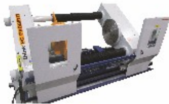
Water jets sliding protection panels.
