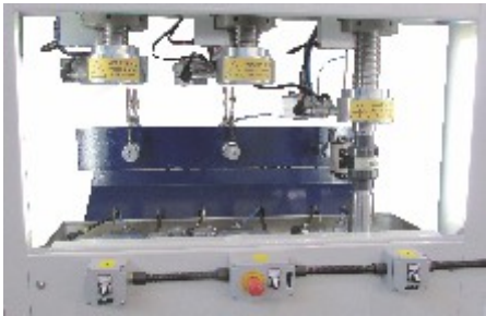
Option for automatic 1/4 turn valve actuator.
