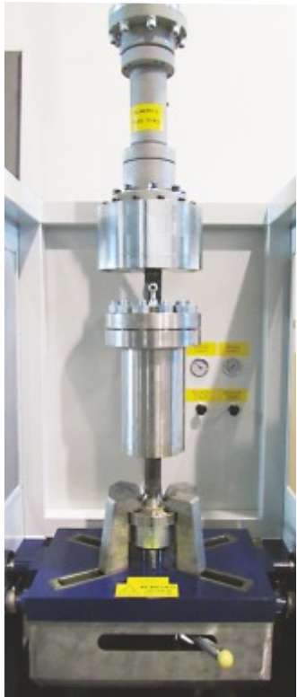
Auto centering claws movement with manual lever
